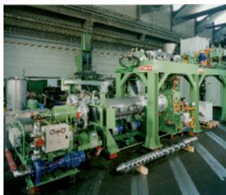
Pomini Compact Compounder CC150/200 with water-ring pelletizer
