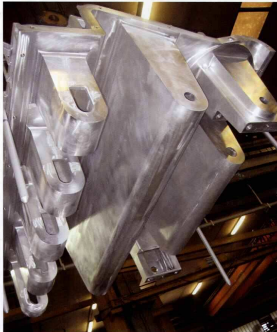
CNC Machined Mold in 4 pieces (a total of 35 aluminum parts joined together) for offshore Buoyancy Module 95x50x36 inches (2421x1270x916mm) - Courtesy of Remcon Plastics Inc.
