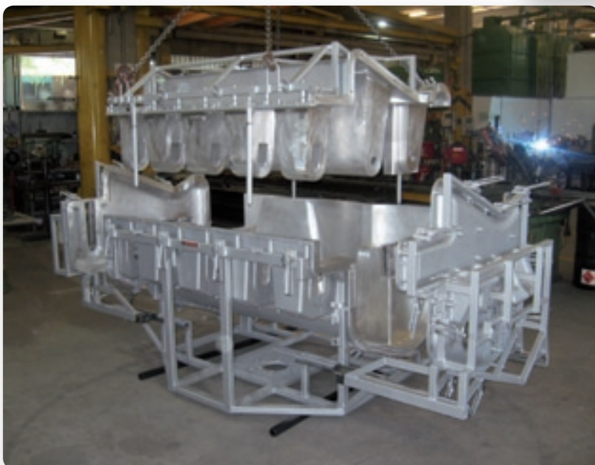
CNC Machined Mould in 4 Pieces (a total of 35 aluminium parts joined together) for Offshore Buoyancy Module 95x50x36 inches (2421x1270x916mm) Courtesy of Remcon Plastics Inc.
