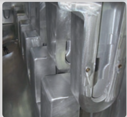
CNC Machined Mould in 4 Pieces (a total of 35 aluminium parts joined together) for Offshore Buoyancy Module 95x50x36 inches (2421x1270x916mm) Courtesy of Remcon Plastics Inc.
