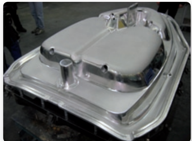
CNC Machined Mould for a Sailing Boat 102x39x23 inches (2600x1000x600mm)
