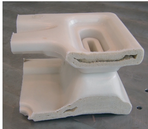
A view of the special Siluma sand reinforced PE core of the Pvaxx pallet
