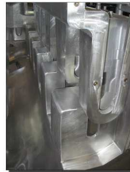
CNC Machined Mold in 4 Pieces (a total of 35 aluminium parts joined together) for Offshore Buoyancy Module 95x50x36 inches (2421x1270x916mm) Courtesy of Remcon Plastics Inc.
