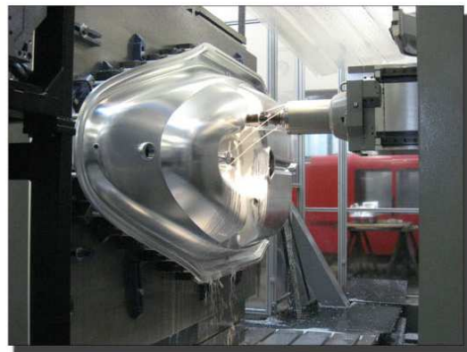
CNC Machined Mold for a Sailing Boat 102x39x23 inches (2600x1000x600mm)
