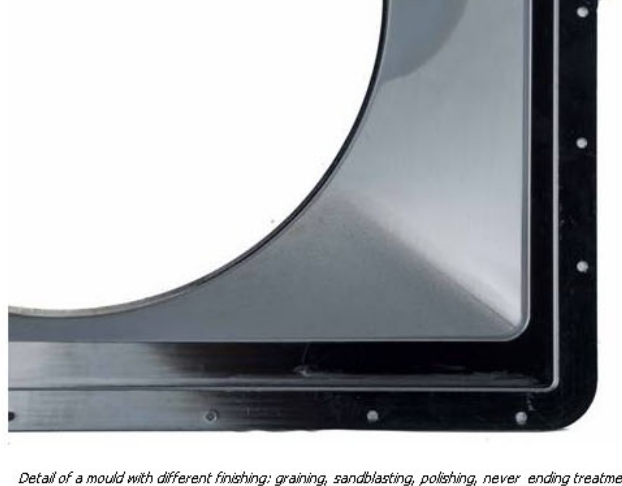
Detail of a mould with different finishing: graining, sandblasting, polishing, never ending treatment.
