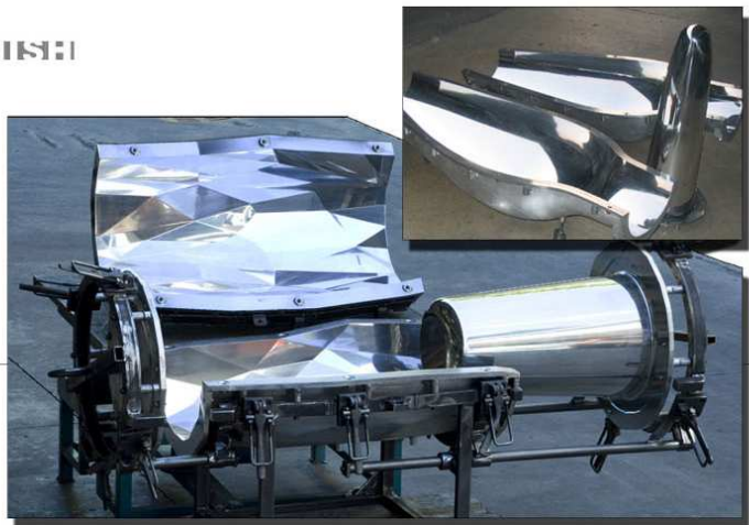
CNC Machined Mold in 4 Pieces (a total of 35 aluminium parts joined together) for Offshore Buoyancy Module 95x50x36 inches (2421x1270x916mm) Courtesy of Remcon Plastics Inc.
